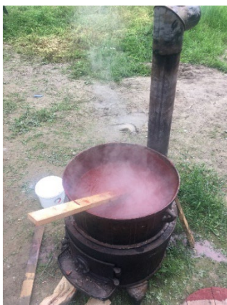
Figure 2. Boiling flour paint. The paint should be stirred continuously.
