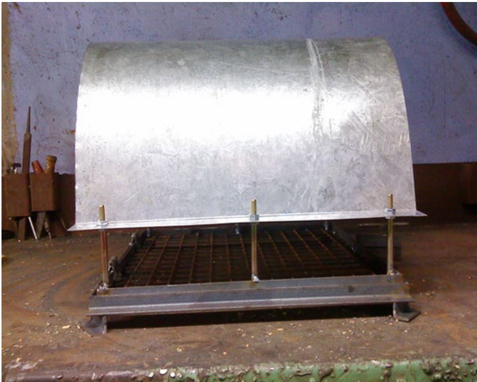
Figure 29. The image shows a cap inspired by 19th-century style but adapted and technically modified by engineer Chico Crafoord to ensure safety, strength, and easy handling when the cap needs to be opened for cleaning. The construction
