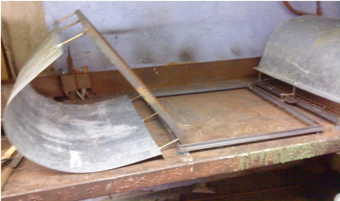
Figure 30. The image shows that the construction can be opened because there are hinges between the frames. Note the angle irons in the corners of the lower frame and the locking mechanism.
